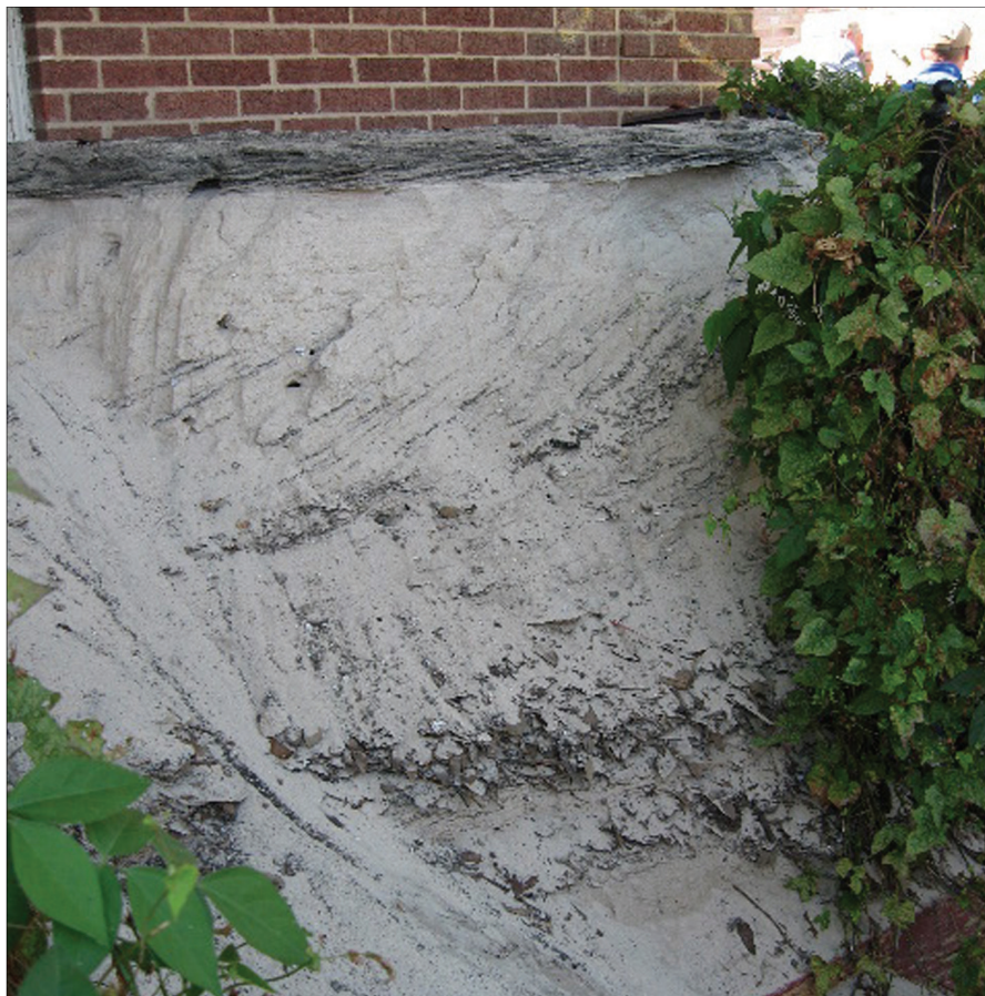
Figure 1: Sand and debris accumulation against a house, caused a levee breach (by Hurricane Katrina in 2005 in New Orleans, USA). People's heads at the back for scale. Photo taken one year after the event. (Photo: S. Warny).
